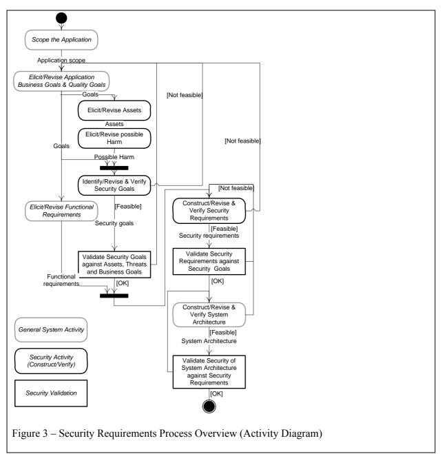
Lines coming out of the bottom of an activity box indicate the successful completion of an activity and carry with them a core artifact into the next activity. Lines coming out of the side of an activity box denote failure and imply the need to iterate back up the process in order to revise an earlier activity. Failure can be one of two kinds: it has been found to be infeasible to create a consistent set of the artifacts that are constructed by that activity; or validation of the artifacts
