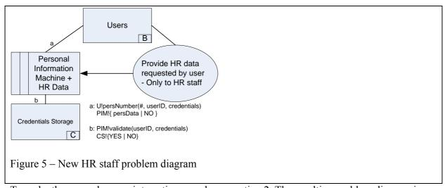
To make the example more interesting, we choose option 2. The resulting problem diagram is shown in Figure 5. The diagram shows that the user is to supply some sort of credentials along with the request for information. These credentials are passed to an external authentication and authorization engine, which answers yes or no. If the answer is yes, then the machine provides the data; otherwise, the data is refused. The corresponding behavior specification is:
