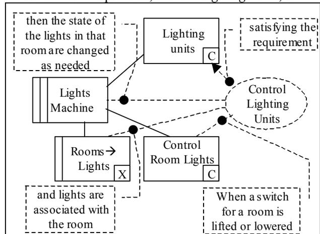
Looking at the diagrams, we see that lifting or lowering a switch causes an event that is a phenomenon shared with the Switch Machine. The machine determines which logical room is to have its lights changed, and is the source of a phenomenon shared with the Lights Machine, as shown in the second diagram. The second machine determines which lighting units are involved, and then is the source of phenomena shared with the appropriate lighting units.
